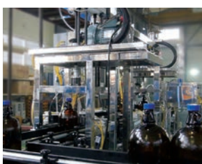
Bottle Filling System 설치가례
